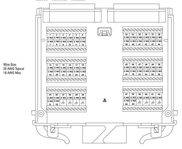
34939A 64-Channel High-Density Form-A GP Switch Module
